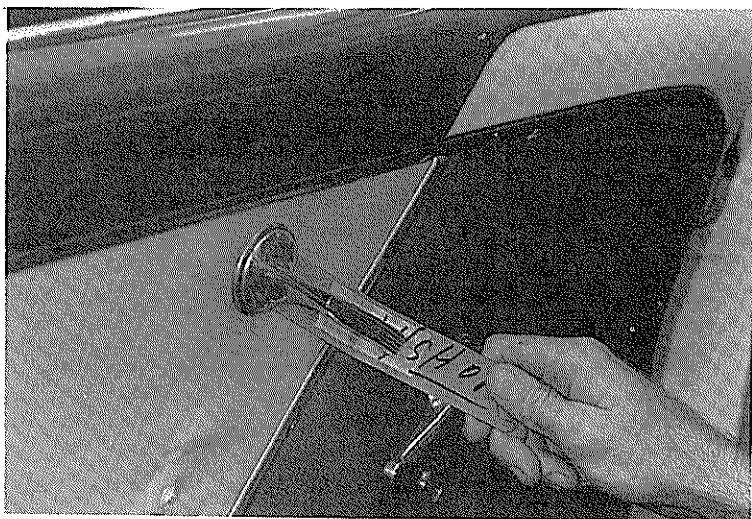
Using the door handle removing tool remove the interior door and window winder handles.
